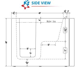
11/2" Bath Drain & Overflow 2" HurryDrain™ Secondary Emergency Drain Power Drain
